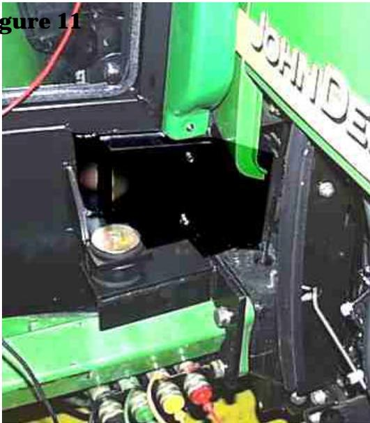
11. Take the left floormat piece that will fit against the bell housing and place it against the left front enclosure shield. Ensure that it fits against the tractor well and glue into place. See Figure 12. Repeat for the right side, and use Figure 13.
