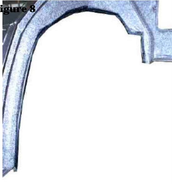
8. Take the 180d O-rubber, and beginning at the bottom of the left side panel where the 90d O-rubber ended, install the O-rubber all the way around to the back of the cab and around the right side until you reach the same point on the right side. Use Figures 7-9 to guide you.
