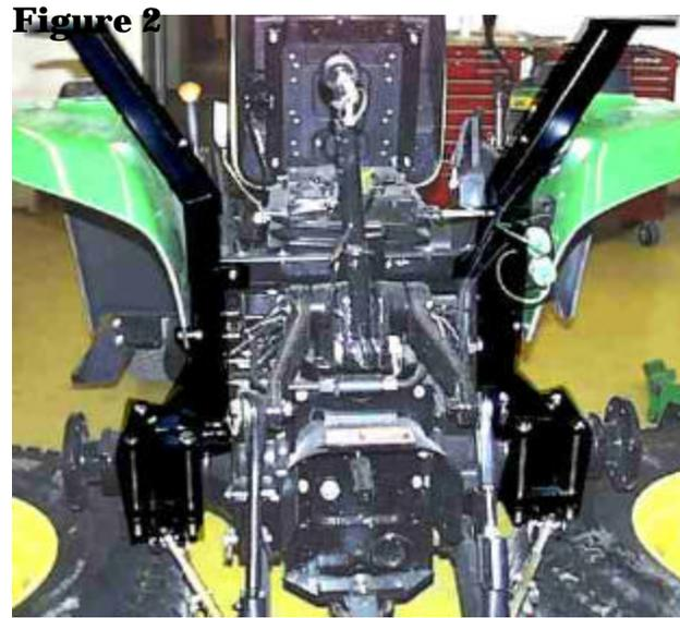
3. If the tractor is NOT equipped with a front-end loader, then use the front bracket spacers provided, otherwise continue with front bracket installation. It will be necessary to remove the top two loader bracket bolts, and the bottom front bolt in order to attach the front bracket. Position the left front bracket onto the loader bracket (or mount spacers) and using the M16x2.0x60 hex bolts and 5/8" lock washers, loosely bolt the bracket into place as shown in Figure 3.
