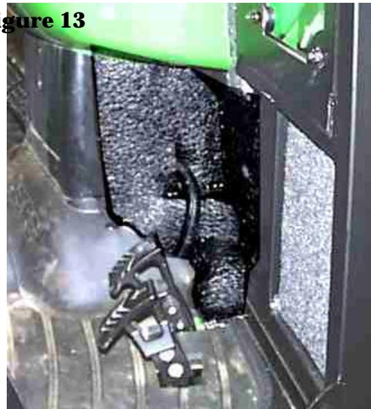
12. Proceed with electrical harness hook-up, locate wires at bottom of A-post. Connect the heavy red wire to 12V. Connect the heavy black wire to tractor ground. Connect the orange wire to a switched source on the tractor.
